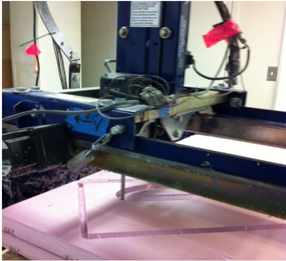
Figure 3: The foam molds for the hulls were fabricated using a CNC Router
