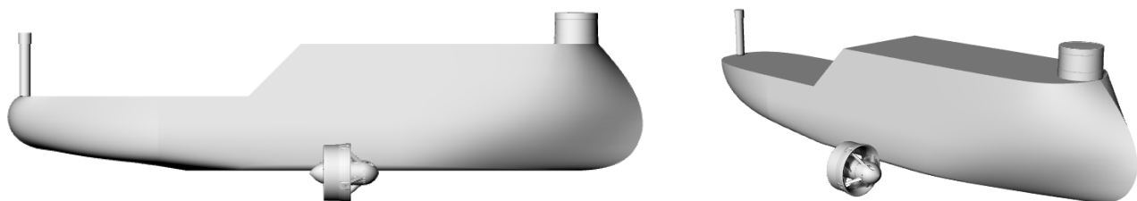
Figure C1. The Orca Hull Renders With Thruster Placement
