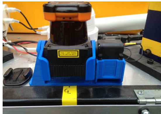
Figure 7: Custom 3D printed LIDAR mount.
