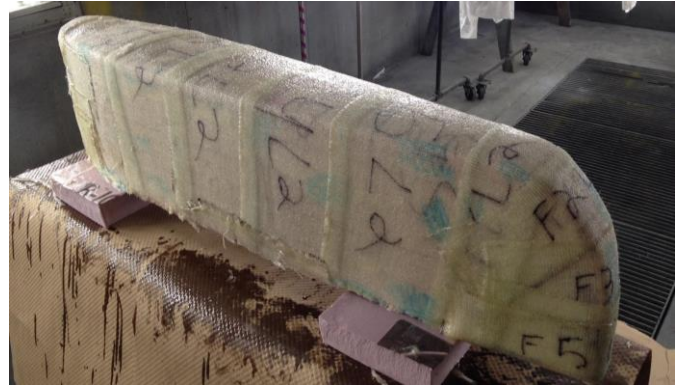
Figure 2: the port sponson during the lay-up stage of fiberglass construction. The thick ridges on the hull are evidence of the overlapping between fiberglass strips.
